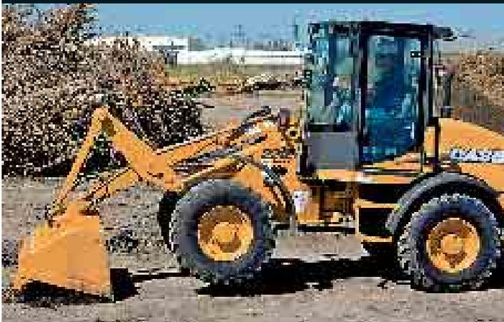
The Case quick coupler, which is standard on all compact E Series wheel loaders, allows for buckets to be completely rotated so that the top of the bucket runs parallel with the ground. This flexibility allows the operator to use the bucket to "pry" the machine out when caught up in difficult, sticky ground conditions. It's also useful for back-dragging material away from foundations, walls or other obstructions.
