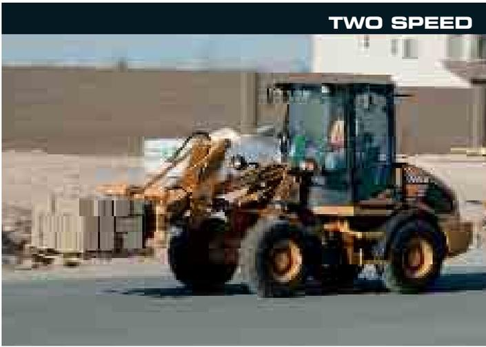
The E Series compact wheel loaders are equipped with an efficient hydrostatic transmission. This provides two speed operation up to 20 km/h on all models. A high speed option on the 121E, 221E and 321E offers a higher speed of 35 km/h. The front axle has a limited slip differential as standard equipment and the rear has limited slip as an option to ensure maximum machine traction when working in difficult ground conditions.
